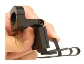
1 - Install your radar detector (RD) onto the mount before attaching to the rear view mirror. To release tension from the spring clip, simply squeeze the tab and the back side of the mount together. This will lower the bottom portion of the spring clip allowing you to slide the RD on and off the
