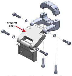
5 - The center-link may be removed if an overall shorter mount length is needed, depending on your rear view miror and desired position for the RD. With multiple adjustments available, you should be able to postion your RD right where you want it. If you are unable to achieve this, be sure to contact us at 1-707-664-8234
